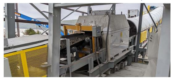
Patented design includes Nuclear Belt Scale
